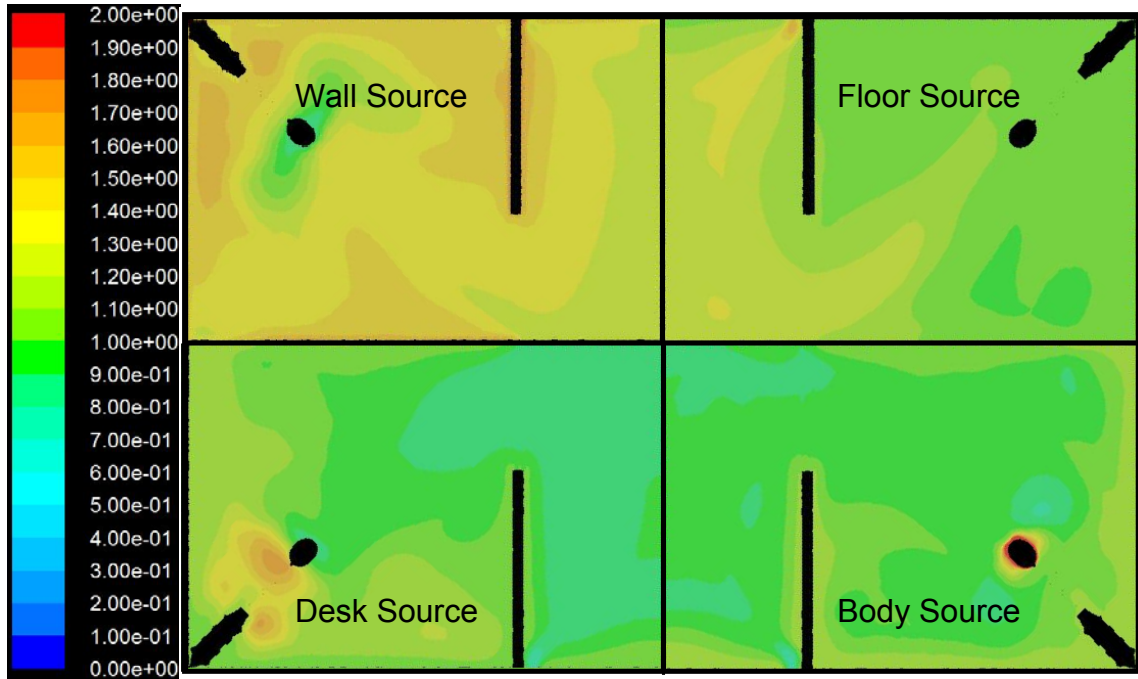
Figure 5.27: Normalized iF along a typical height for a seated person for a conventional ventilation system.
